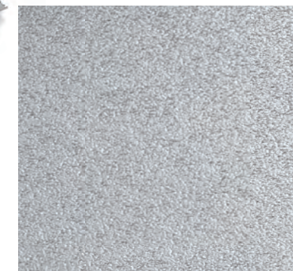
Leather structure reduces visibility of scratch marks
